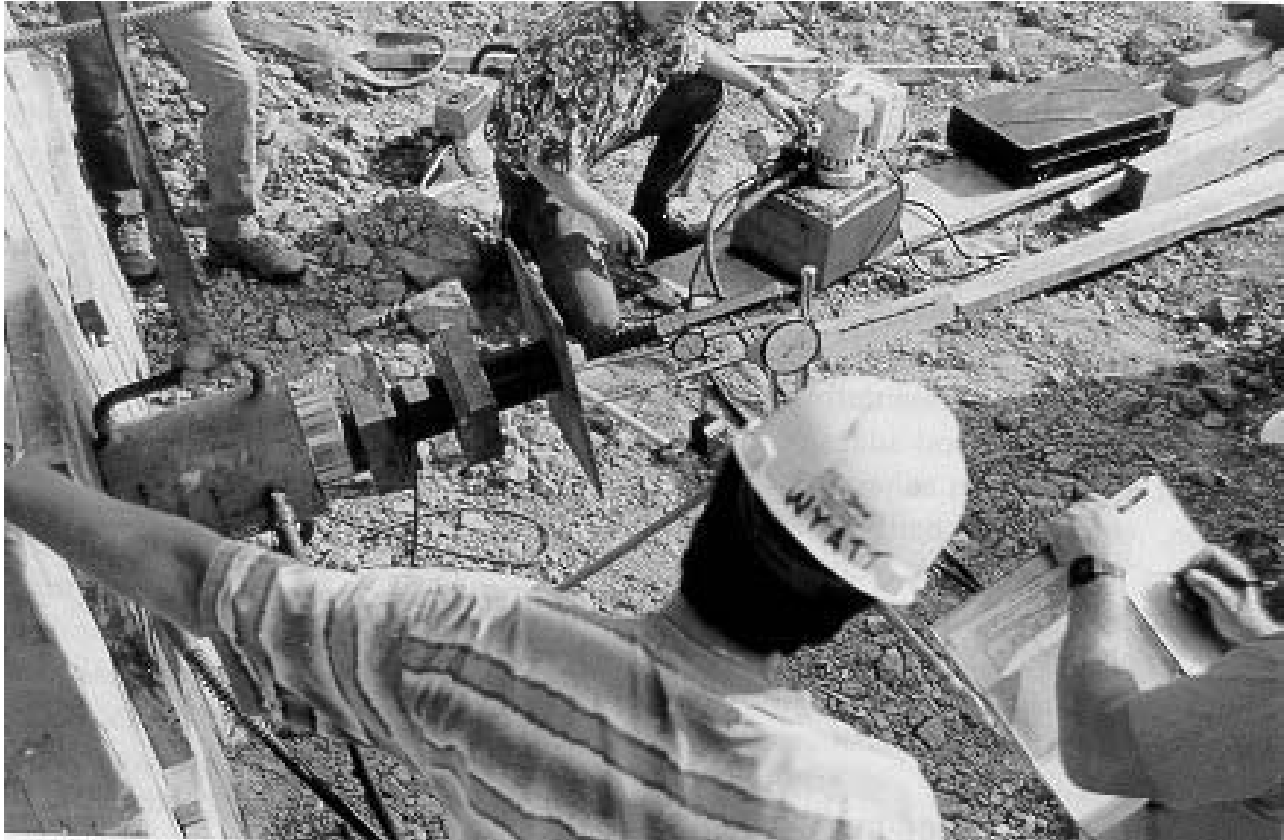
Figure 8.1: Soil Nail Load Testing Setup.
