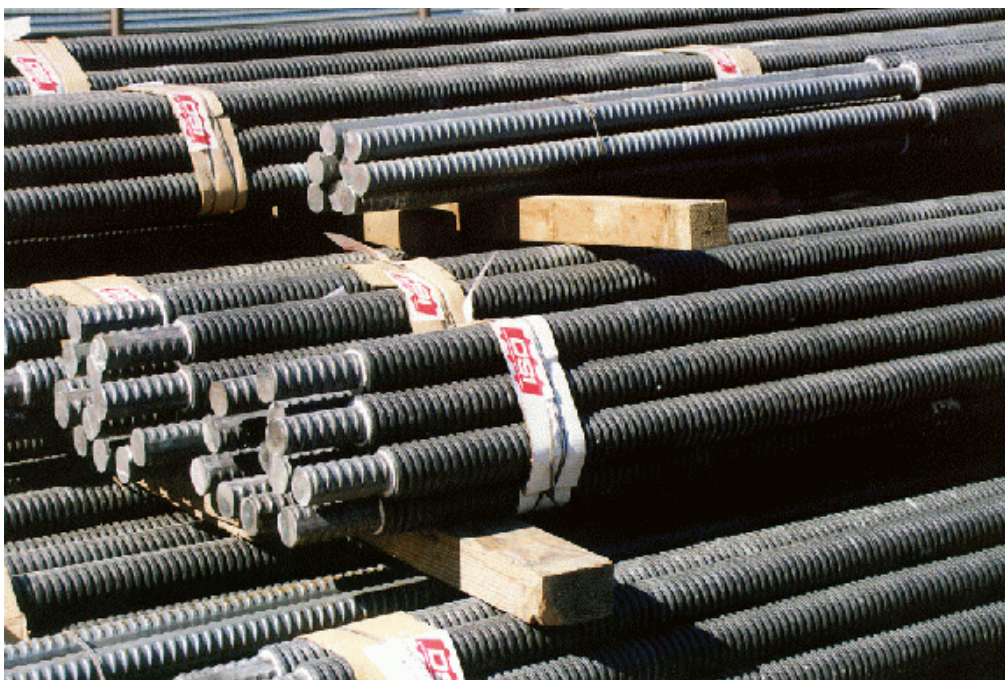
Figure 8-4. Double Corrosion Protected (Encapsulated) Reinforcing Steel.
